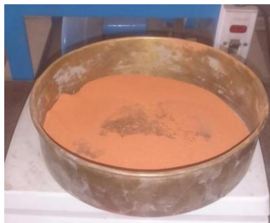
Figure 2.1: Brick dust after sieve analysis
